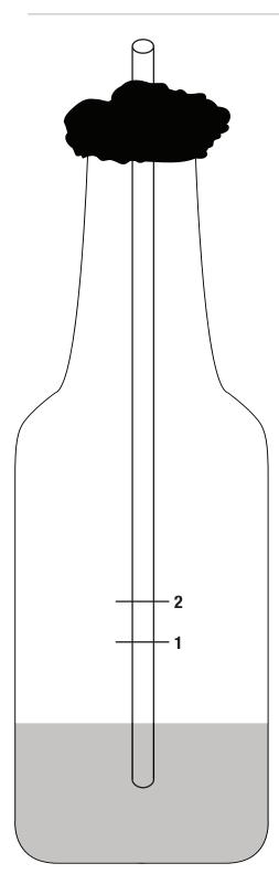
It's time to observe thermal expansion and contraction! How will the indicator liquid behave in different environments and at different temperatures?
